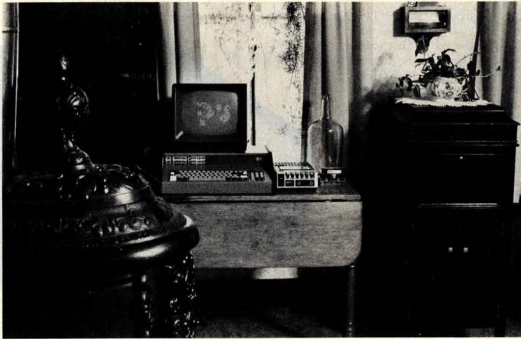
The SOL-20 in a New England parlor context, obviously enjoying life. The entire system fits on one table with a video monitor on top of the computer and an audio tape recorder for mass storage to the right.
